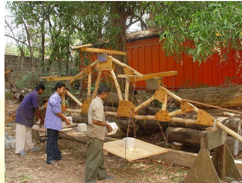
Fig.3 Bamboo truss while testing
